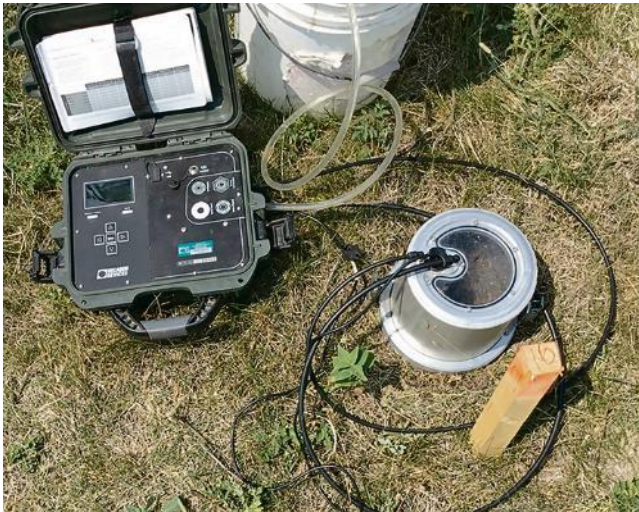
Measuring water infiltration rates under continuous and adaptively managed rotational grazing systems. Photo from Timm Döbert.
