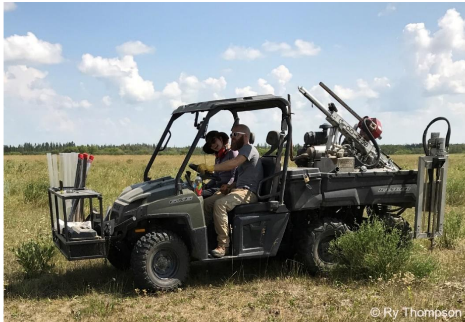
Researchers take 1 m deep soil cores using a quad-mounted hydraulic soil sampler as part of the AMP project. Photo by Ry Thompson.
