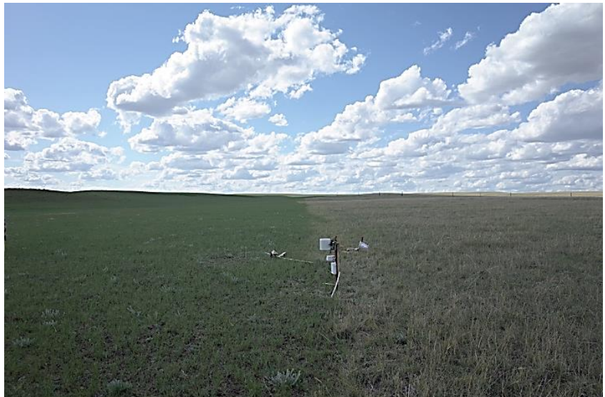
A weather station sitting on the boundary between burned (left) and non-burned grassland (right), in the year following the wildfire.
