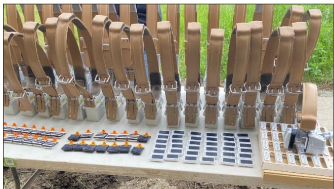
Left: Different technologies being tested at Kinsella Research Ranch in 2022. Back: LOTEK GPS Collars™ (Canada); Front Left: GPS eartags from GPS Collars AS™ (Norway); Front Right: GPS eartags from CeresTag Pty Ltd™ (Australia).
