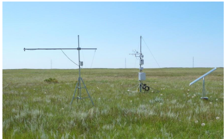
Figure 1. Eddy covariance measurements and surface reflectance measurements at the Mattheis Research Ranch. Photo from Ran Wang.
