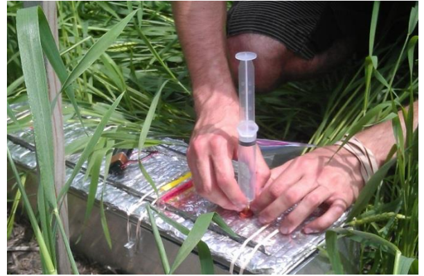
Collection of air samples for greenhouse gas emissions studies using a static chamber. Photo by Ferrah Fatemi.
