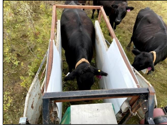
GEM system was used to quantify CH 4 and CO 2 from cattle grazing on open rangeland
