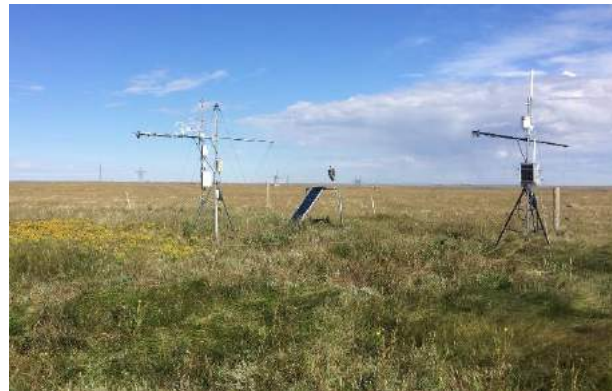
A CO 2 flux tower at the Mattheis Ranch where one methane sensor will be installed.
