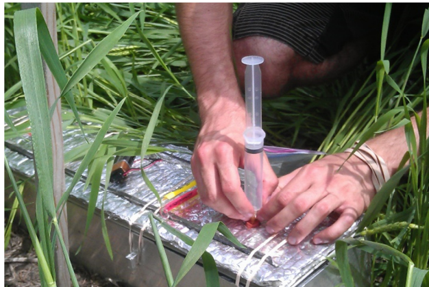
Collection of air samples for greenhouse gas emissions studies using a static chamber. Photo: Ferrah Fatemi.
