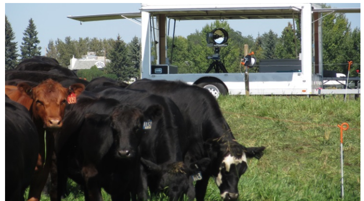
Figure 2. Measuring CH 4 using Open path Fourier Transform Infrared Spectrophotometers (OP-FTIR), Lacombe Research Centre. Photo by T. Flesch.
