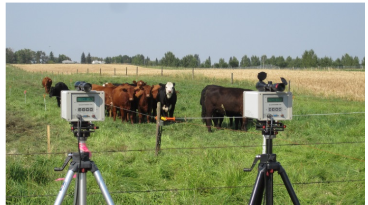
Figure 1. Measuring methane (CH 4 ) using Boreal laser at the Lacombe Research Centre. Photo by V. Baron.
